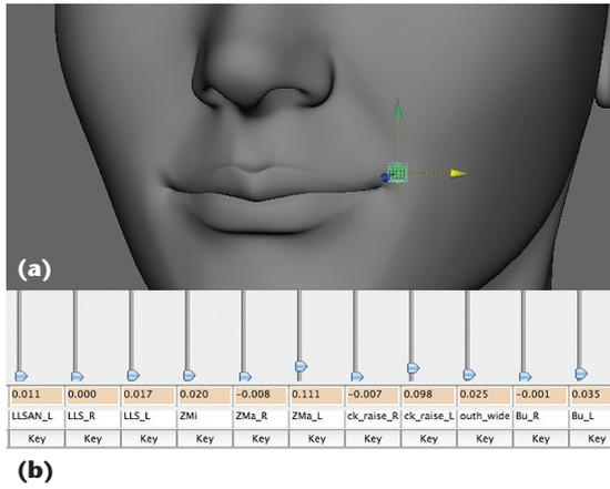
**Figure 6. The relationship between direct movements and slider movements. (a) Direct movement of a single vertex creates (b) many subtle slider movements. However, the converse is also true: a single slider movement in some cases equals multiple direct manipulations. Both approaches are desirable.**
