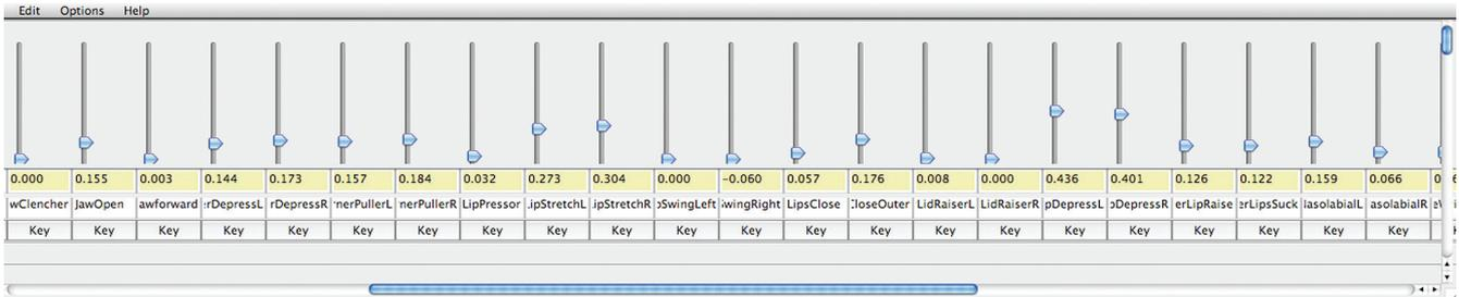
Figure 2. A portion of the blendshape slider interface for a professionally created model (the complete set of sliders doesn't fit on the computer display). The model has more than 100 sliders.
