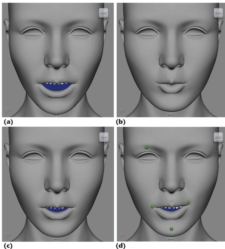
**Figure 7.** Using direct manipulation to make local adjustments on whole-face expressions. The whole-face (a) “ah” and (b) “oo” visemes created in advance. (c) A weighted combination of these two expressions. (d) The result of local direct manipulation.
