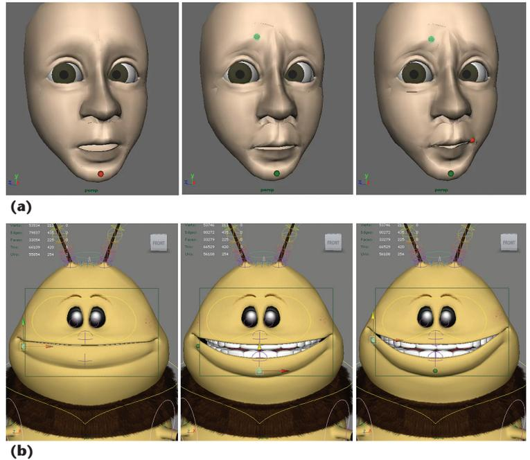
**Figure 3. Screenshots of our system in operation. (a) A blendshape model posed by direct manipulation rather than traditional slider weight editing. (b) Control over a smile's shape by direct manipulation of several vertices. The figures are screen captures of the Maya program interface and are low resolution owing to hardware rendering.**
